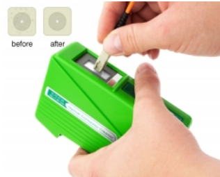
cleaning of fiber optic connectors
