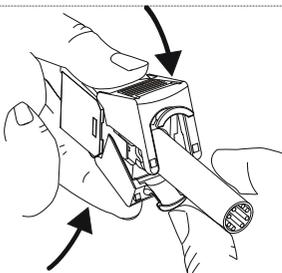
Close up the wings towards each other and push down both sides for secure connection.
