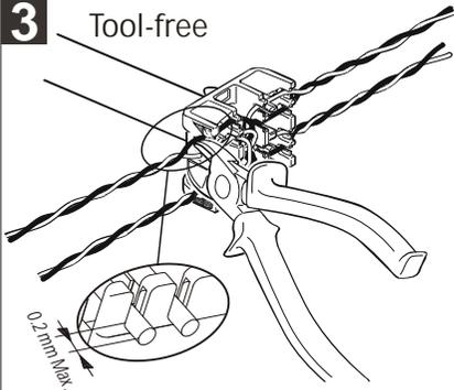
Insert the wires through the cap and seat the wires in the correct slots according to T568A or T568B. Trim the wires flush with the cap. It's recommended that the tip of the wires is no longer than 0.2 mm.
