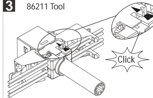
Insert the wires through the cap and seat the wires in the correct slots according to T568A or T568B. Match with the black triangle and align the cap with IDC until it clicks as shown.
