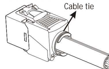
Wrap the drain wire around the shielded holder and tie up the cable.
