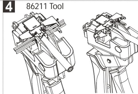
Use the 86211 tool to terminate and cut 4-pairs of wires, simultaneously finishing the installation.
