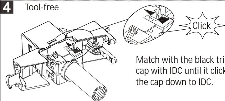
Match with the black triangle and align the cap with IDC until it clicks as shown. Press the cap down to IDC.
